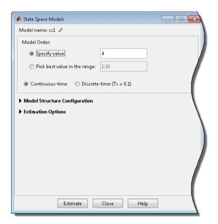
To access the redesigned Linear Model Refinement dialog box, in the System Identification Tool, select **Estimate** > **Refine Existing Models**.
