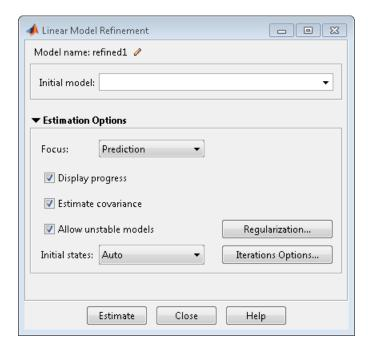
The initial model must be in the Model Board of the System Identification Tool or a variable in the MATLAB workspace. This model can be a state-space, polynomial, process, or transfer function model.
